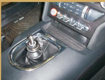
**19** Install the Boomba Racing shift knob (sold separately). If shift pattern does not line up heat it up with the hair dryer. Line up the shift knob with the car.
