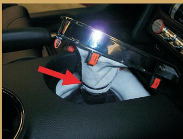
**18** Snap the boot assembly into place and install the storage tray liner.
