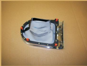
**17** Line up the boot assembly and pull the cloth over the shifter. Secure it in the top groove with the zip tie.
