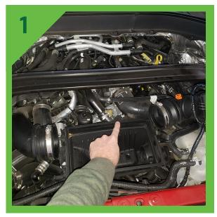
Remove the OEM filter and airbox in order the access the diverter valve underneath.
