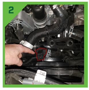
Locate the OEM diverter valve on the charge pipe. Remove the diverter valve and unplug the wiring harness.
