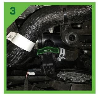
Install the Boomba BOV adapter between the charge pipe & the diverter valve using the provided hardware. Reconnect the wiring harness.
