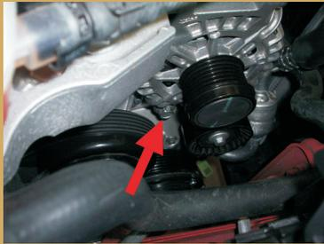
**22** Remove the top alternator screw and the nut.
