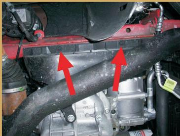
**15** Move the belt tensioner arm and remove the serpentine belt.
