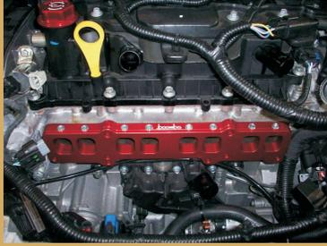
**27** Reinstall the intake manifold and secure it with the provided longer bolts.
