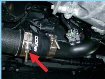
**17** Disconnect the vacuum line and the AT sensor. Remove the nut holding the charge pipe to the transmission.
