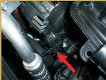
**21** Remove the bottom alternator screw.
