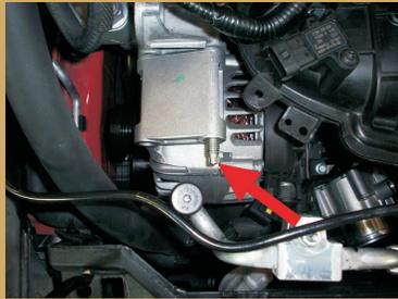
**24** Remove the intake manifold's bolts. Two M8 and four M6 bolts.
