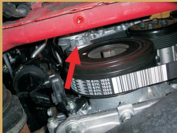
**16** Loosen the intake pipe clamp.
