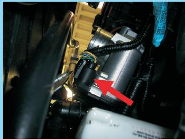
**20** Disconnect the alternator wire harness.
