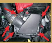
Snap off the air supply duct from the latch.
