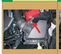
Loosen the air pipe clamp and remove the air pipe.
