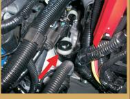
Reinstall the air supply tube, the vent line and the air filter box. Tighten all hose clamps and bolts. Reconnect the MAF sensor.
