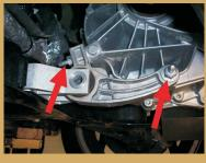
Remove the wishbone rear bolt.
