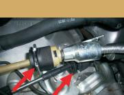
Reinstall the shifter cables.
