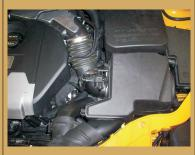
Reinstall the battery tray and the air box. Tighten the hose clamps. Reinstall the battery cover, the air filter and the filter cover. Reconnect the MAF sensor connector.
