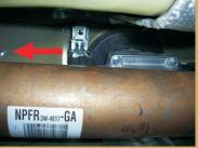
Push the shifter assembly up and align the mounting studs. Secure the bracket to the body.
