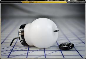
TO REALIGN, REMOVE THE KNOB & USE A SMALL ALLEN KEY TO PUSH OUT THE GEAR PATTERN CAP.
