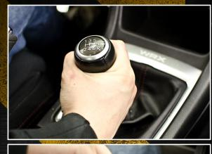
REMOVE OEM SHIFT KNOB BY UNSCREWING IT COUNTER-CLOCKWISE.
