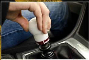
SCREW ON BOOMBA SHIFT KNOB AND TIGHTEN IT UNTIL IT IS SNUG.
