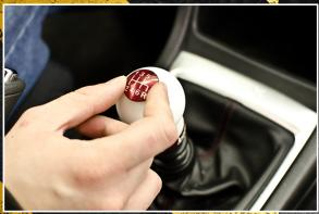
LINE UP THE GEAR PATTERN CAP AND PUSH IT INTO PLACE.
