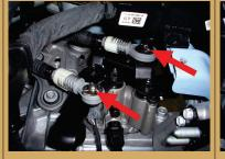
Secure the shifter cable bracket to the transmission. Super glue the bottom bushings to the bracket.
