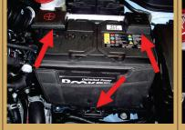
Remove the spring clips. Remove the
