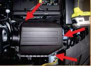
Remove the screw holding the wire
